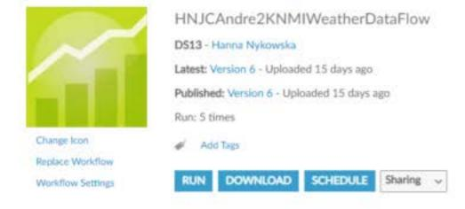
Download and unpack zip files containing historical data from weather stations in the Netherlands. The zip files contain a single txt file and there is a separate zip file for each weather station. The workflow downloads all the zipfiles as temporary files and then unions the text files into a one dataset.
